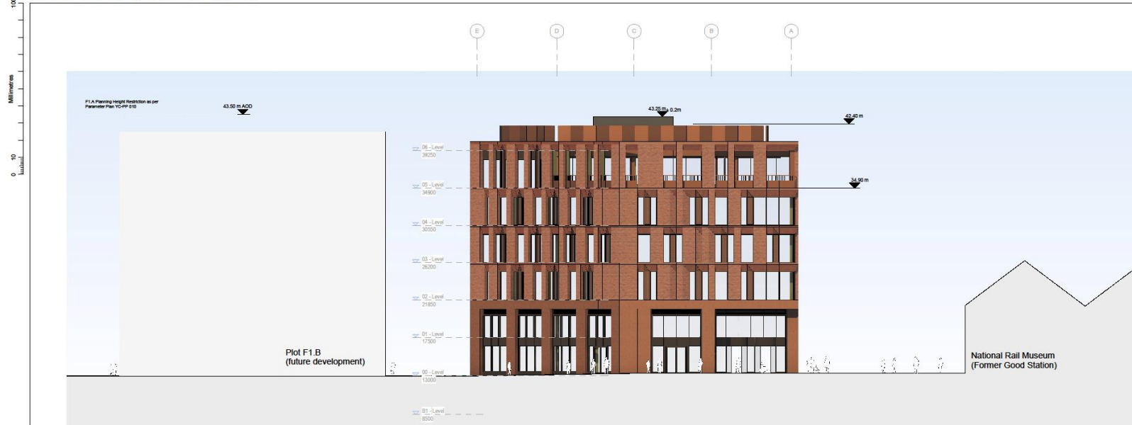
1 | East Elevation - Planning 012202 SCALE 1: 200
